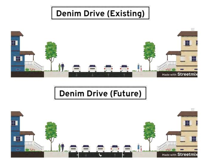
The cross-sections above shows how Denim Drive could be converted from a 4 lane facility to a two-lane road with a center turn lane and on-street parallel parking. This would increase pedestrian safety and comfort while still providing adequate room for vehicular traffic.
